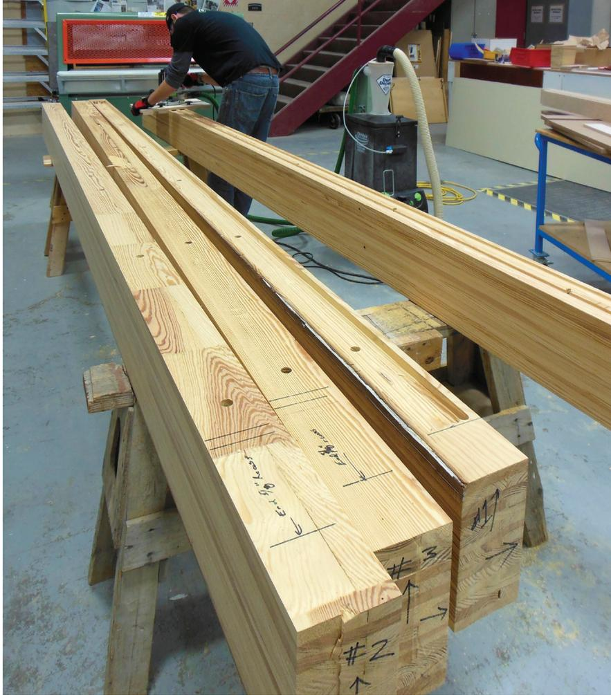
glue-laminated White Oak members represented critical structural elements used in the hulls of wooden minesweepers that were built for the United States Navy by Peterson Builders, Inc., of Sturgeon Bay, Wisconsin.
