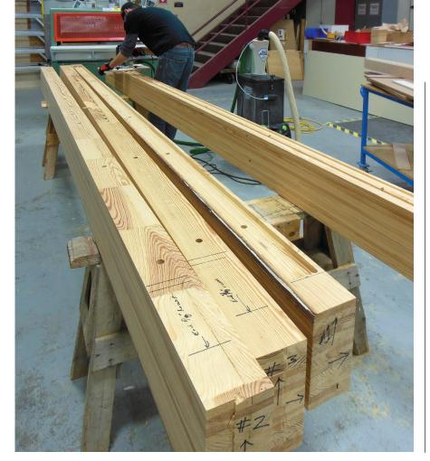
glue-laminated White Oak members represented critical structural elements used in the hulls of wooden minesweepers that were built for the United States Navy by Peterson Builders, Inc., of Sturgeon Bay, Wisconsin.
