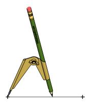
2. Spread and Lock the divders to a distance that is more than half the length of the line.
