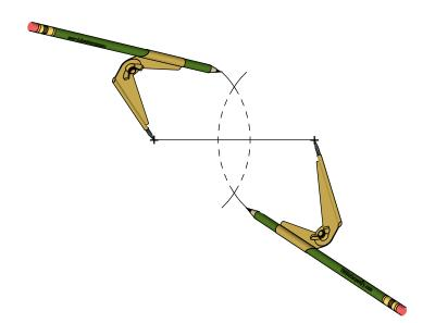
3. Keeping the dividers locked, draw arcs through the center of the line from each endpoint.
