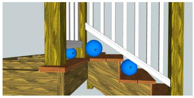
One solution for correcting these problems is installing a second newel post near the nose of the first tread. But that means two extra newel posts (additional costs), and a very tight spacing between newel posts, barely enough room for two balusters!
