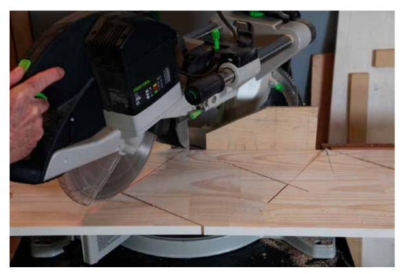
Finally, flip the board one last time and cut the top where the back of the stringer flushes out with the back of the newel post.
