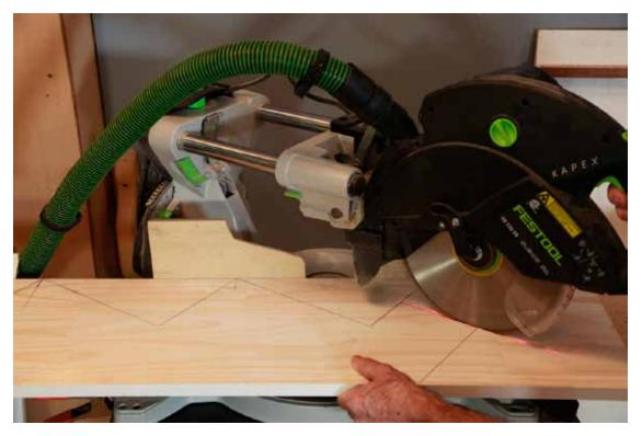
Next, swing the saw to 34 degrees and cut the risers, working from the top down.
