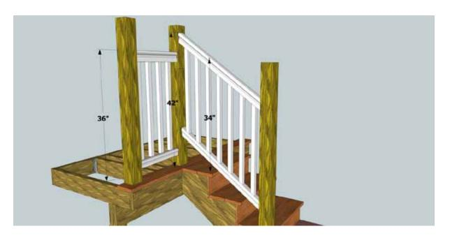
While that approach simplifies hanging the stringers—because connectors can be attached directly to the rim joist—it complicates newel post and handrail design.
