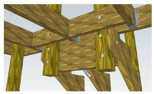
hanger. Besides, by running the outside stringers to the back of the newel posts, bolts could pass through the stringer and the newel post in the opposite direction (see left), reinforcing the upper newels so they'd easily handle 200 lbs of concentrated load—another IRC code requirement.
