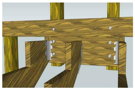
Someone else chimed in and suggested we extend the outer stringers flush with the back of the newel posts, otherwise they'd be fastened too close to the end of the hanger: Even if we used Simpson's new stringer hanger (LSCZ), the nails would be right at the edge-grain of the wooden
